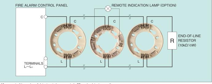
• Max, permissible number of detectors to be connected : 30 smoke detectors per line
